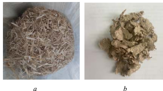
Fig. 3. Cellulose extraction from industrial hemp: a – technical hemp before cooking; b – unbleached pulp from technical hemp
