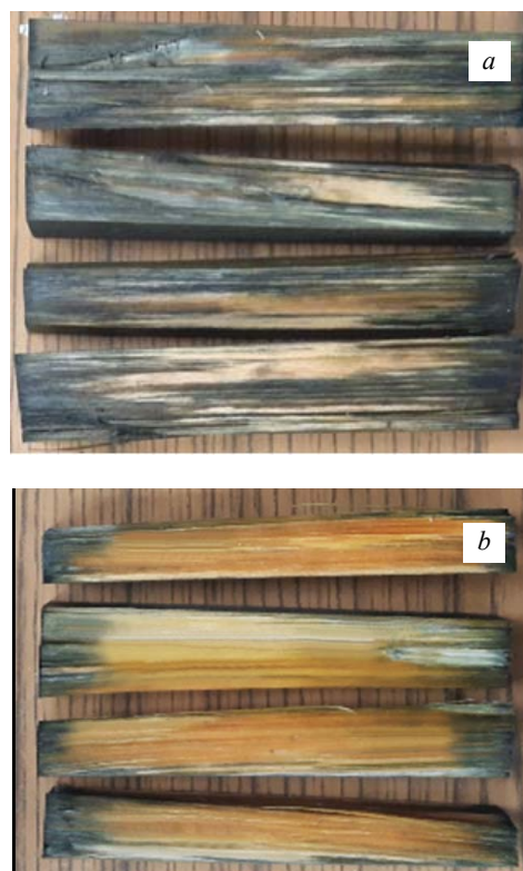
Fig. 2. Samples of wood after impregnation without waterproofing the ends: a – microwave-treated; b – untreated microwave (control)
