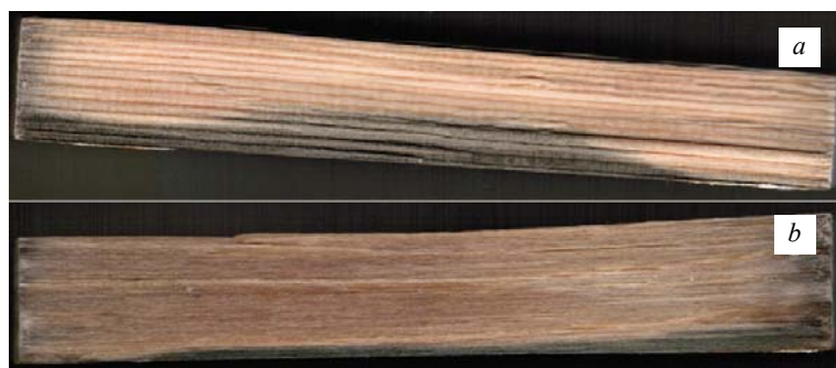
Fig. 8. Fragments of wood samples treated with microwaves and impregnated with closed ends: a – radial direction; b – tangential direction
